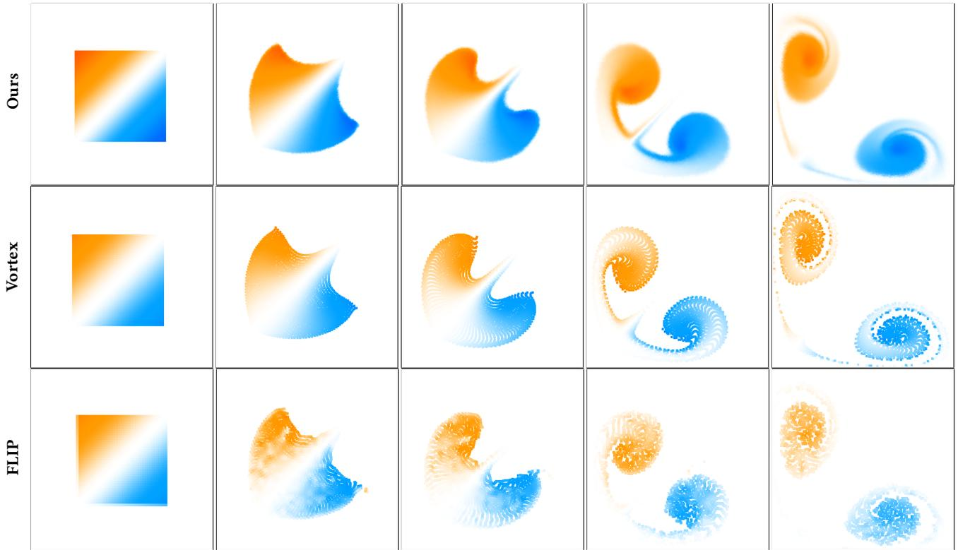
Fig. 10. **Comparison with standard solvers:** Left to right,  $t = 0, 1, 2, 5, 10$  seconds. Our method (top) produces results that are consistent with the vortex particle (middle) and hybrid FLIP (bottom) baselines. Colors visualize the signed vorticity at each (particle) position.
