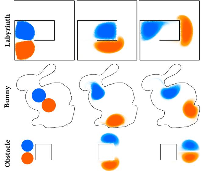
Fig. 4. **Free-slip boundary conditions:** Left to right,  $t = 0, 5, 10$  seconds. Two vortices propagating in a maze (top), a flow inside a more complex bunny-shaped boundary defined using a signed distance function (middle), and vortices flowing around a solid obstacle in a periodic domain (bottom).
