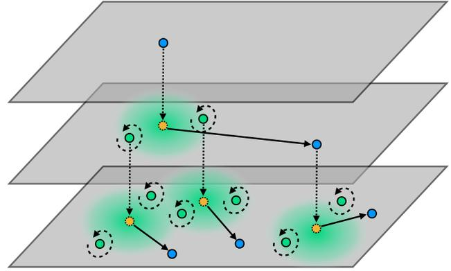
Fig. 3. **Exponential complexity:** Applying our basic recursive formulation leads to exponential cost as, starting from a point of interest (blue, top), we must trace back for every random sample generated during the Biot-Savart approximation (green), leading to an exponential branching factor.
