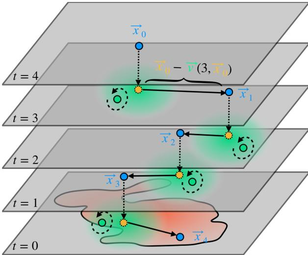
Fig. 2. **MC backtracing:** To compute vorticity at a point and time of interest (in blue, top  $t = 4$  layer) we project the point back to the previous time step (in yellow) and compute its velocity with our Biot-Savart estimator. To do so, we generate random samples around the projected points (green), recursively computing their vorticity. Once computed, we advect along the velocity to the next position and repeat until we reach the initial condition.
